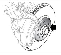
Clean any rust or dirt from the contact surfaces between the wheel and brake disc
