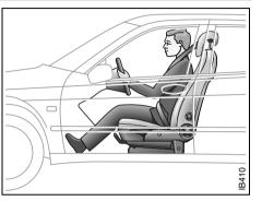
Correctly positioned safety belt
