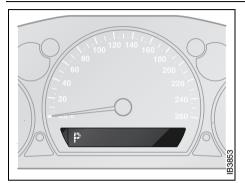
Selector-lever indicator on main instrument panel
