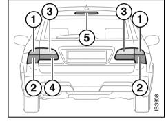
Rear light clusters, 9-5 SportCombi 1 Direction indicators 2 Stop lights and taillights 3 Reversing lights 4 Rear fog light 5 High mounted broke light
