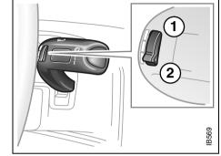
Control for setting wiper delay 1 Long delay 2 Short delay
