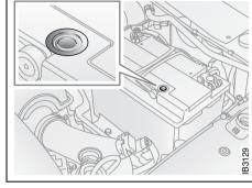
Checking the battery electrolyte level. Dark or green level indicates the correct fluid level. Battery should be changed if indicator is light
