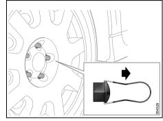
Removing the plastic wheel bolt caps
