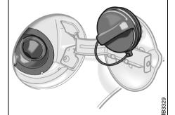
When refueling, hang the fuel cap inside the fuel door
