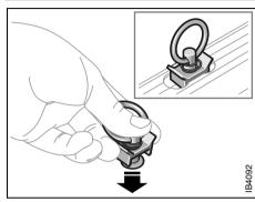
Cargo tie down eye **\*** mounted on the longitudinal rails **\***
