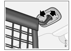
Attaching the cargo net to the roof
