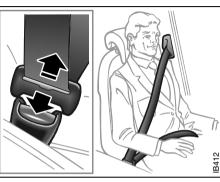
Press the red button to release the belt
